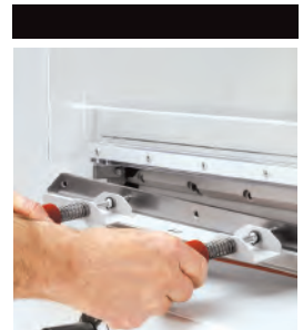
The blade changing device covers edge of blade for safe handling.
