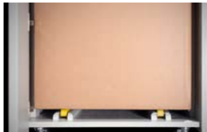
Conveyor of rollers on each side allows for easy removal of the 50 gallon waste container.
