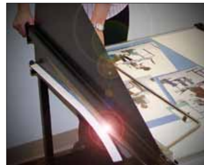
Metal safety shield prevents hands from being in the wrong place.
